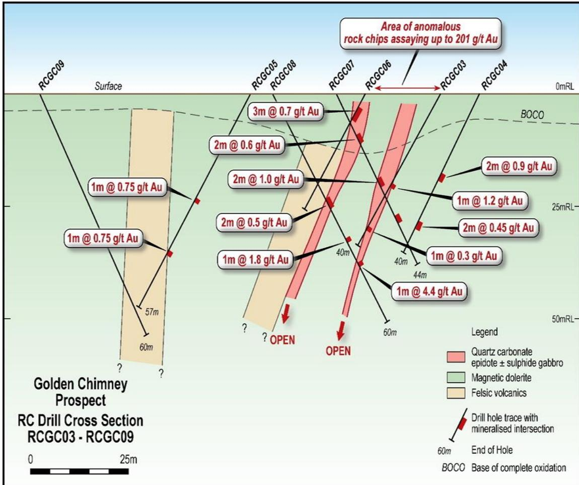
Figure 11. RC drilling cross section for several historical drill holes at the Golden Chimney Prospect. See Figure 10 for location.
